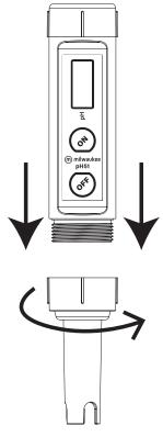
Make sure the gaskets are in place before screwing back the ring.
